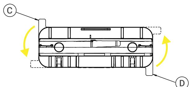
**EN:** Insert the adapter into the track, so that the mechanical key (A) in the adaptor matches the groove (B) in the track. Rotate of about 90° the levers of the two cams (C and D) until they reach the locking position.
