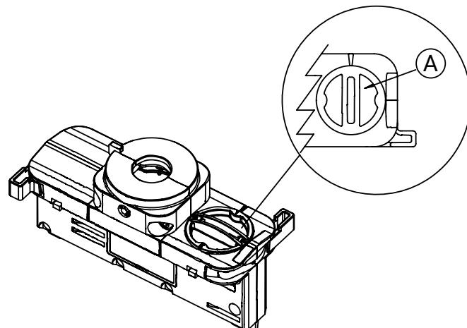
**EN:** When the track is connected to a three-phase system it is possible to select the phase (L1, L2 or L3) to distribute the single luminaires in the system, by means of the proper selector (A) of the adaptor.
