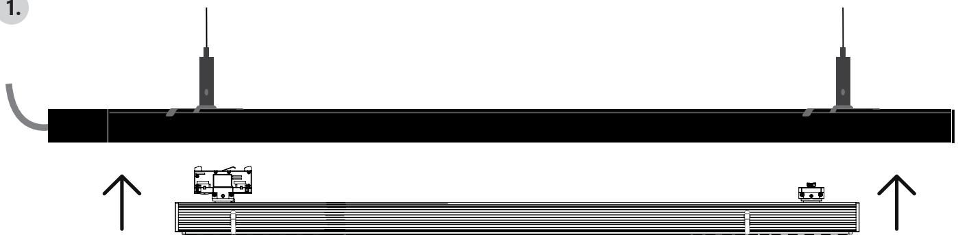
**EN:** Insert the luminaire into the track.
