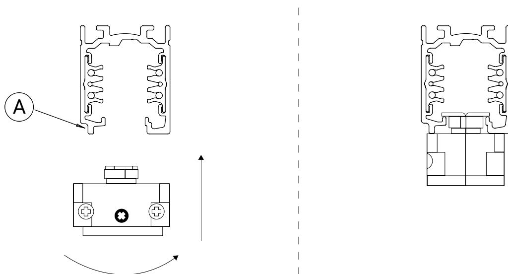
**EN:** Insert the mechanical adapter into the track, indifferent of the position of the mechanical key (A), and rotate it 90°.
