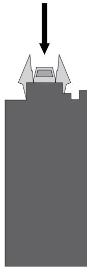
**EN:** Push down on the upper mechanical key (located at both ends of the luminaire) using a long slim flat head screwdriver.
