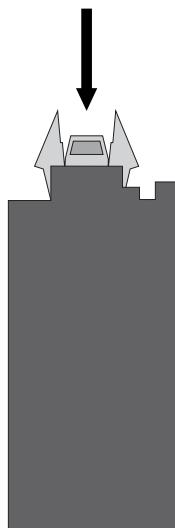
**EN:** Push down the upper mechanical key (located at both ends of the luminaire) to release the lower mechanical key.
