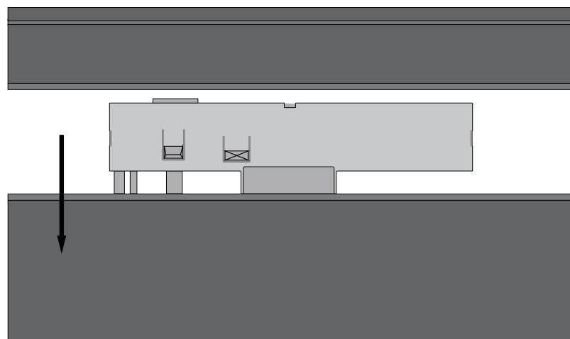
**EN:** Make sure that the adaptor is fully released from the track before performing other actions.
