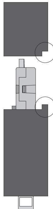
**EN:** Before inserting the adaptor into the track make sure that the mechanical key of the luminaire matches the groove in the track.
