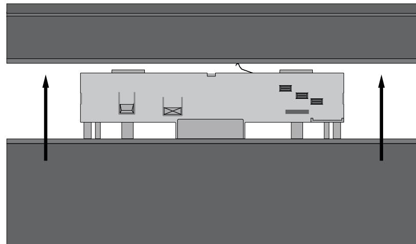
**EN:** Insert the adaptor into the track and press on the luminaire until they are close together.
