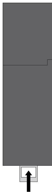
**EN:** Push up on the lower mechanical key (located at both ends of the luminaire) to secure the luminaire on the track.
