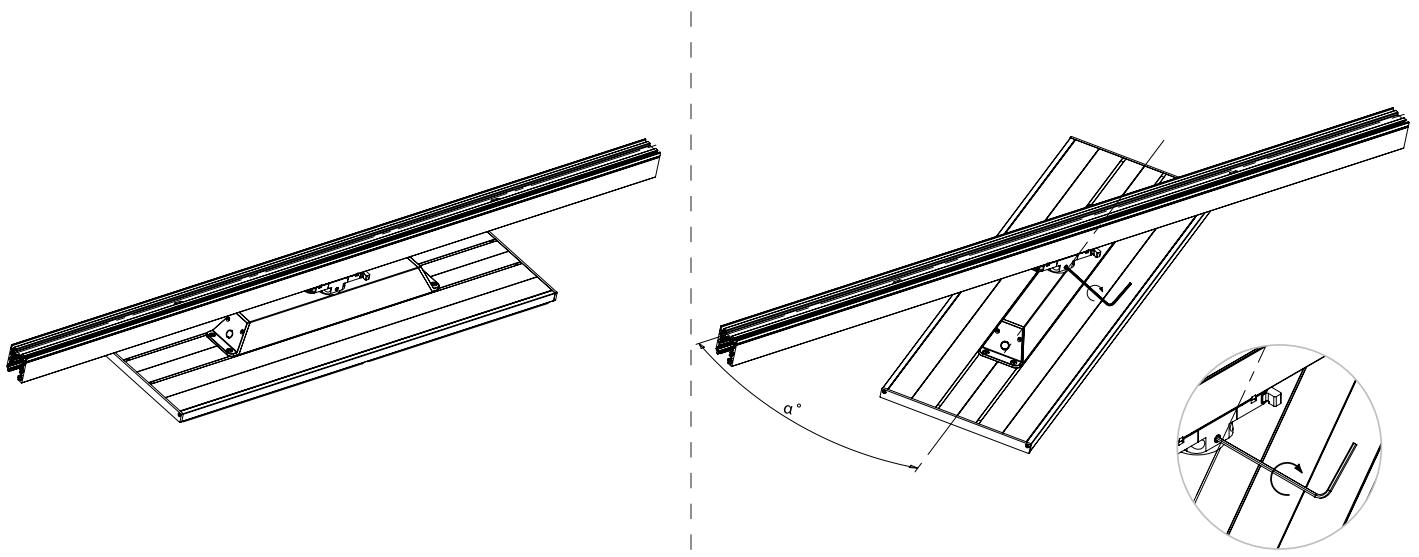
**EN:** Adjust the luminaire to the desired angle ( $\alpha^\circ$ ). Tighten the locking screw with a 2mm allen wrench.
