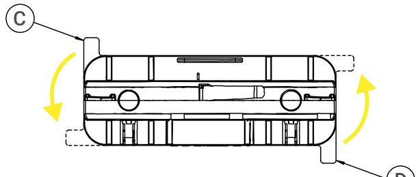
**EN:** Insert the adapter into the track, so that the mechanical key (A) in the adaptor matches the groove (B) in the track (pic.1.3). Rotate of about 90° the levers of the two cams (C and D) until they reach the locking position (pic. 1.4).
